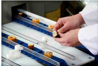
**Image 2:** The ratio of the aperture to the size of the product is an essential consideration as sensitivity is measured at the geometric center of the aperture.
