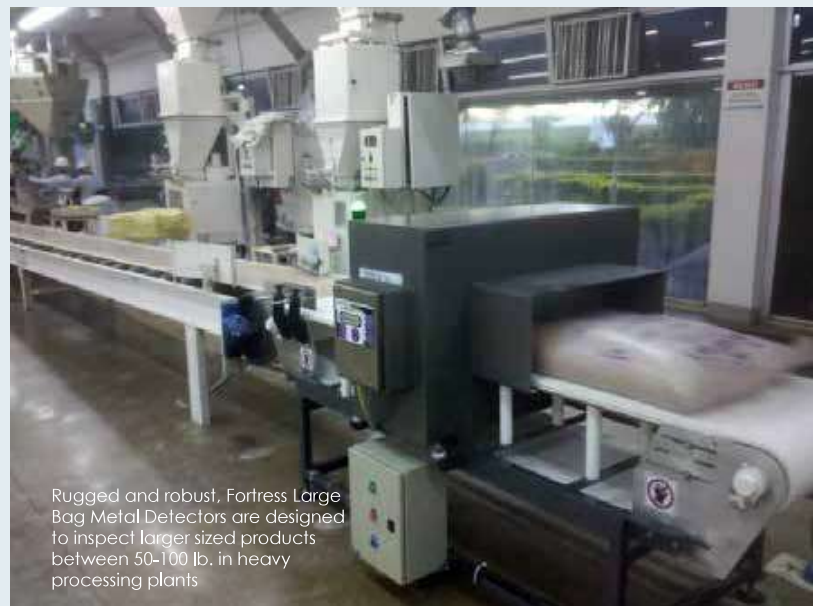
To optimise efficiency, heavy-duty conveyors, gravity inspection and Lab QA metal detectors can be added to bulk processing lines
