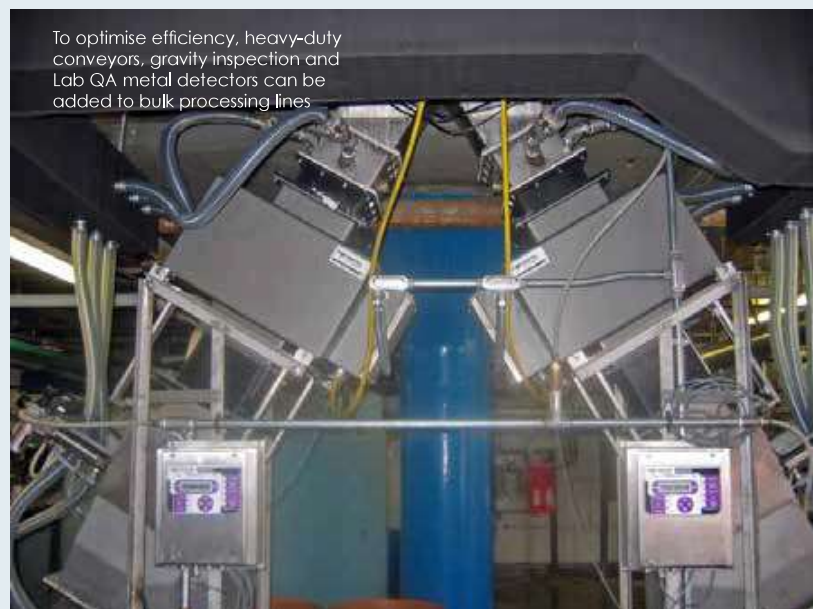
Rugged and robust, Fortress Large Bag Metal Detectors are designed to inspect larger sized products between 50-100 lb. in heavy processing plants
