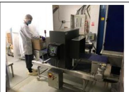
**Image 1:** OCM's Fortress Stealth metal detector checks up to 400kg of tablets per hour
