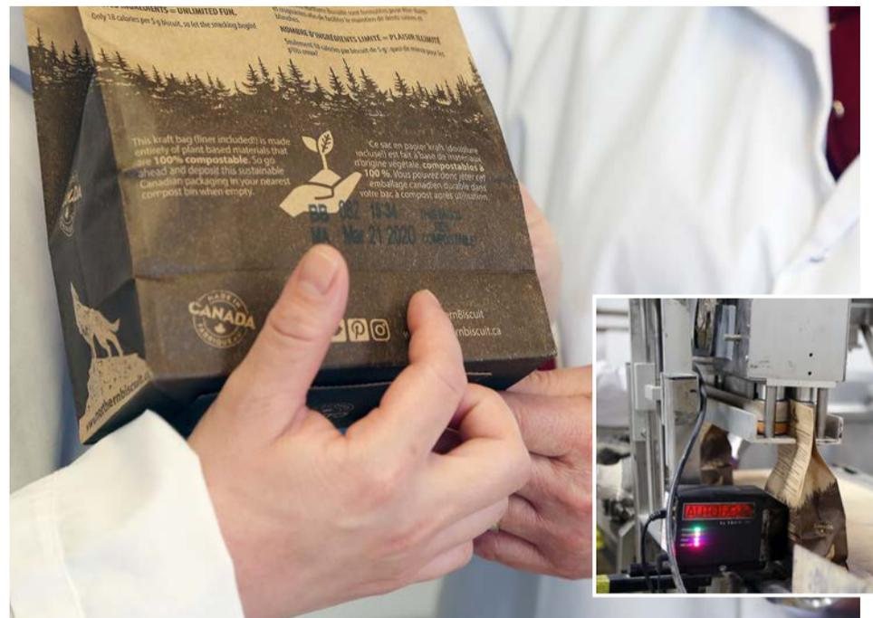
The AutoPilot at work, quickly and quietly applies the coding data to the back of a bag of Northern Biscuits brand healthy dog treats at the fast-growing Northern Pet Foods facility in Concord, Ont.
