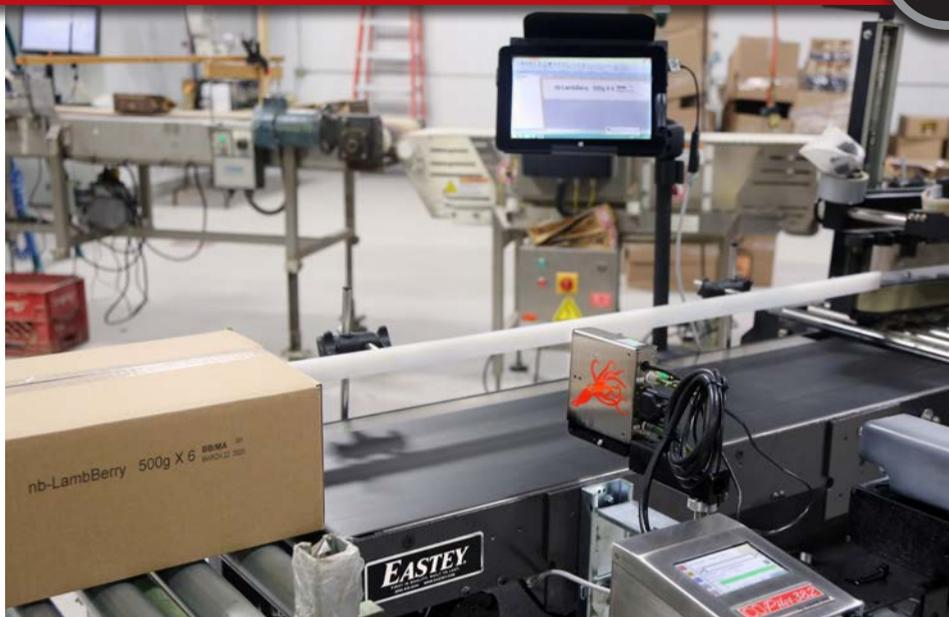
A CoPilot 382 manufactured by Squid Ink is mounted on an Eastey EC1248 conveyor applying product identification data after exiting an Eastey SB-2 Taper unit, which were all supplied to Northern Pet Products by Dependable Marking Systems.
