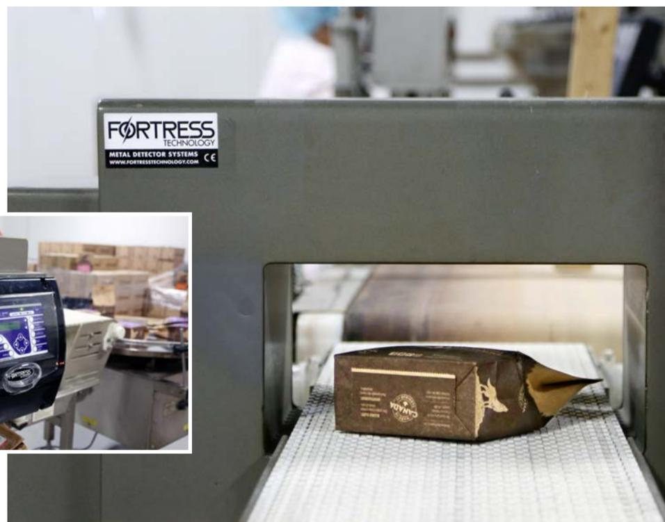
The bakery uses a Stealth metal detection unit manufactured by Fortress Technology, providing Northern Pet Products with an additional comfort level regarding the safety of its healthy dog biscuits, thanks to the system's highly-sensitive digital signal processing tech.
