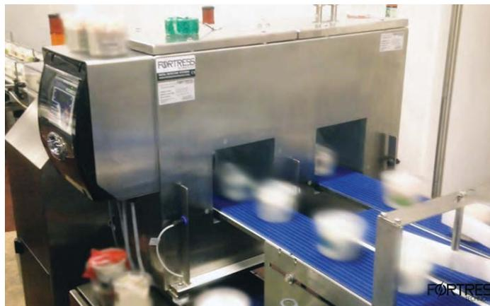
The multiaperture, multilane metal detector cuts the overall equipment footprint by 50 per cent and TCO (total cost-of-ownership) by over 65 per cent.
