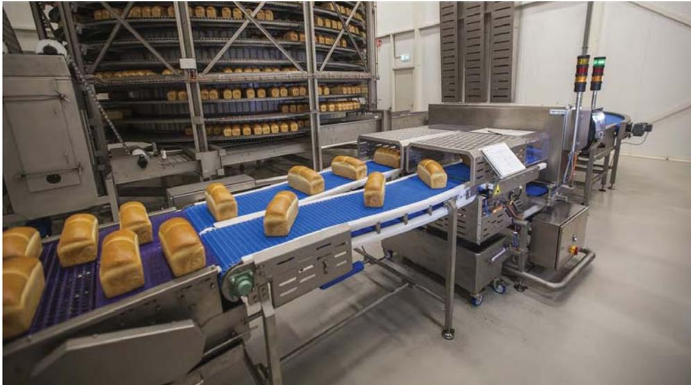
Dutch bakery Borgesius inspects 14,000 fresh loaves of bread per shift on its twin aperture system.
