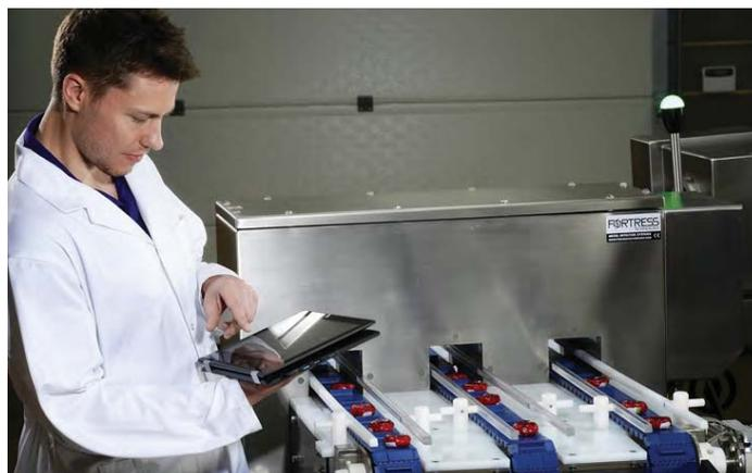
All lanes run independently to increase production efficiency, with all the collected data analyzed and monitored side by side.
