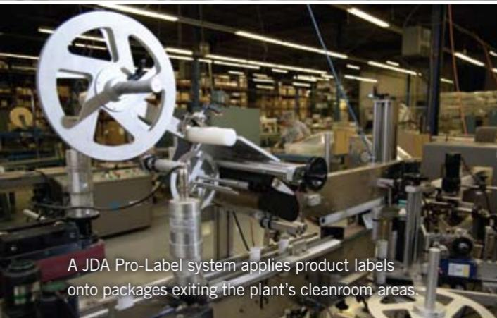
A JDA Pro-Label system applies product labels onto packages exiting the plant's cleanroom areas.
