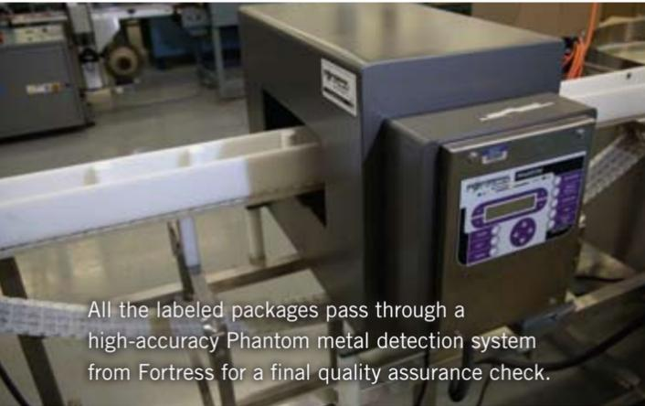
All the labeled packages pass through a high-accuracy Phantom metal detection system from Fortress for a final quality assurance check.
