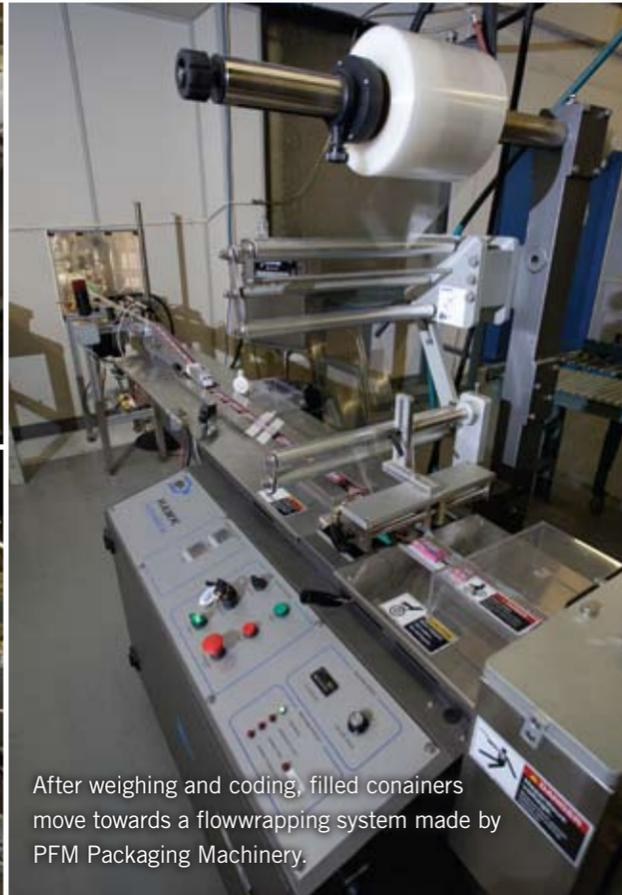
After weighing and coding, filled containers move towards a flowwrapping system made by PFM Packaging Machinery.
