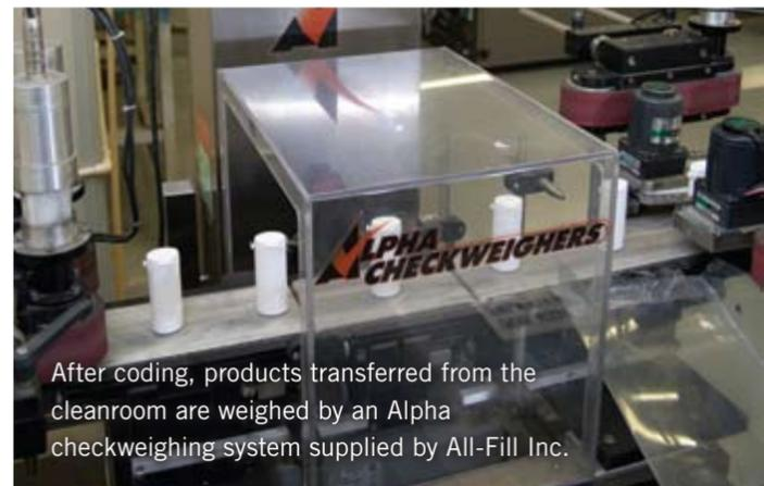
After coding, products transferred from the cleanroom are weighed by an Alpha checkweighing system supplied by All-Fill Inc.
