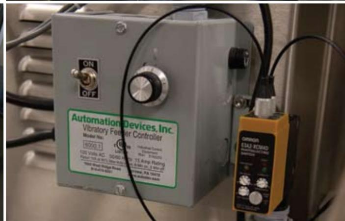
The vibratory feeders system working with the JDA Pro-Cap 5000 capper incorporates several Omron photoelectric switches.
