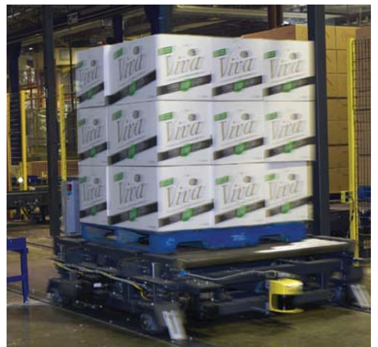
The Yum Yum plant utilizes an innovative shuttle conveyance system, specifically manufactured for it by Wulftec/M.J. Maillis Group, that greatly increases its production flow.
