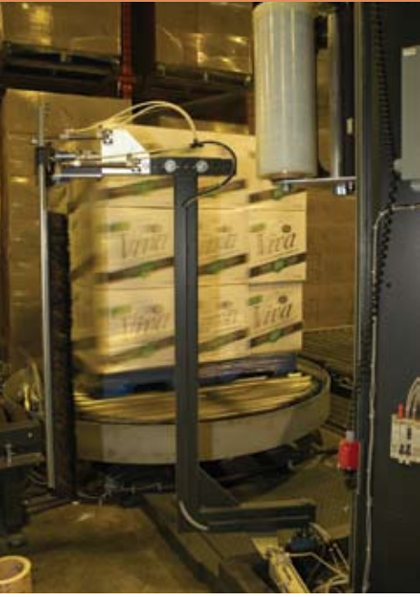
Purchased through Techno Pak Packaging Systems, a Wulftec WCA-150 stretchwrapper securely binds a pallet of Viva Veggies snack chips together.
