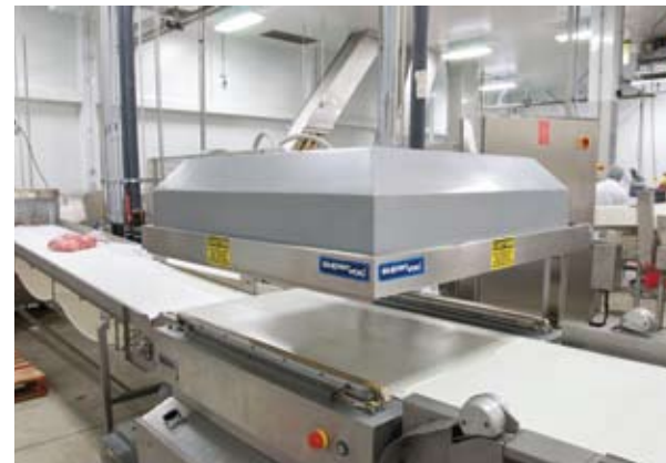
A new Reiser SuperVac chamber machine uses a high-pressure sealing system for a strong, reliable seal.
