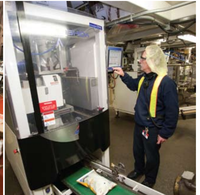
Packaging machine operator Bruce Haines makes on-the-fly adjustments to the fully-automatic Douglas Machine case-packing line that utilizes high-performance suction cups to ensure gentle placement of bags of potato chips into the corrugated shipping boxes.
