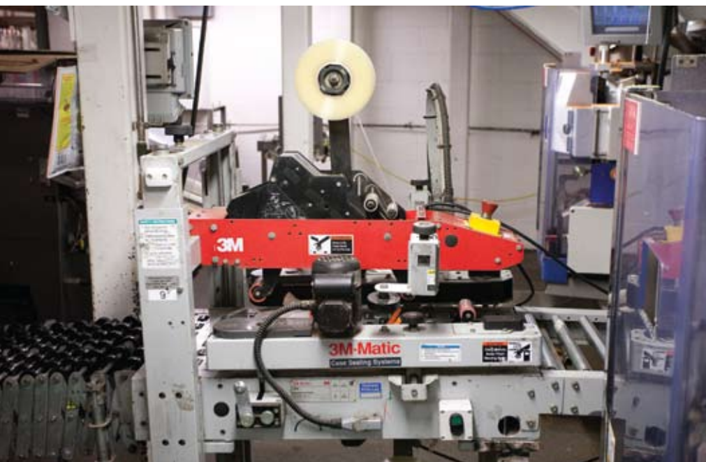
One of several 3M-Matic case-sealing machines from the 3M Company used to secure bags of potato chips inside the corrugated shipping cases.
