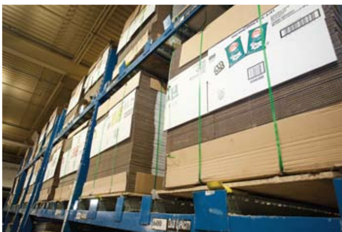
Strapped stacks of palletized pre-printed corrugated boxes, manufactured by Mitchel-Lincoln Packaging, are stored on steel racking in the Cambridge plant's vast warehousing area near the shipping docks.
