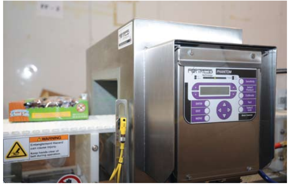
Cartons of School Safe nut- and peanut-free product pass through a Fortress Technology Phantom metal detection system to ensure optimal products safety.
