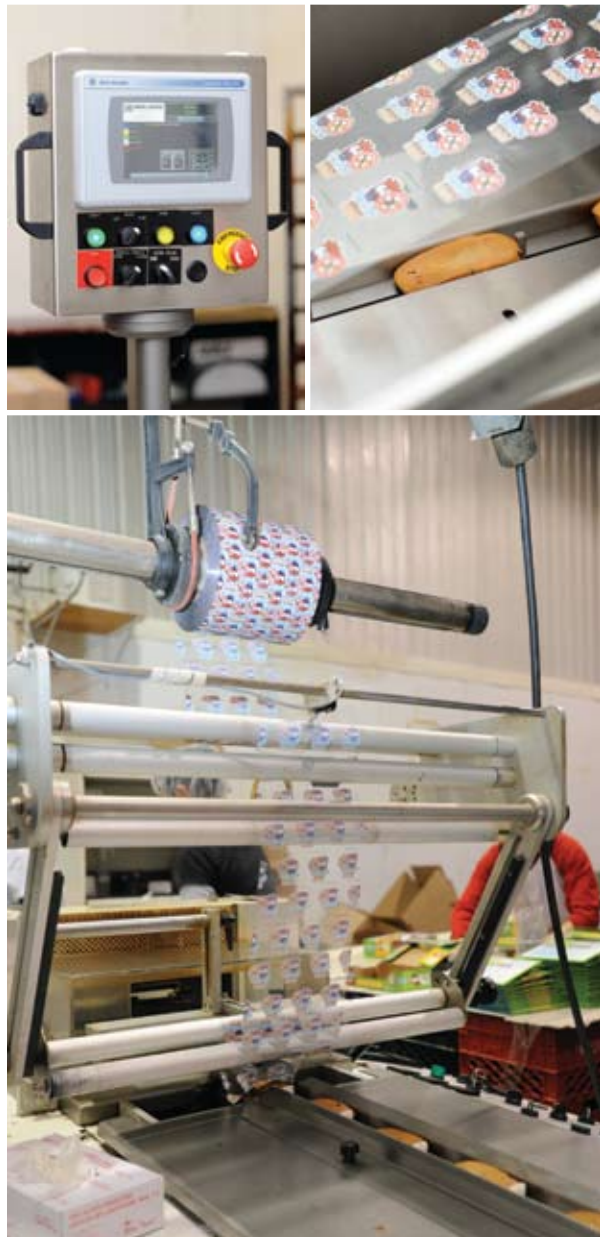
Controlled by a Rockwell Automation Allen-Bradley PanelView Plus 700 (top left) operator panel, a Campbell Wrapper Heritage horizontal flowwrapper with film supplied by Vista-Pak is used to individually seal in the freshness of its School Safe baked products.
