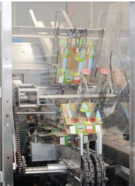
A Consolidated Technologies cartoner opens the Cascades paperboard folding cartons and places the individually-wrapped School Safe snacks inside.
