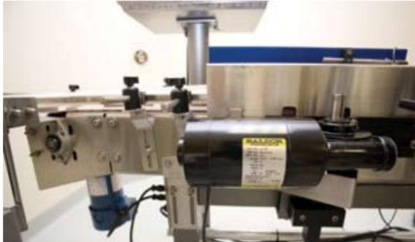
A ¼-horsepower Baldor Electric motor powers a Speck-Tech Systems conveyance line in one of Orbus Pharma's packaging rooms.
