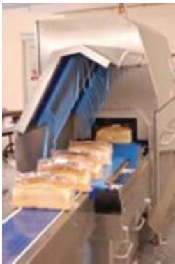
Protective lead curtains on x-rays must be well maintained and cannot come in to contact with unpackaged food.
