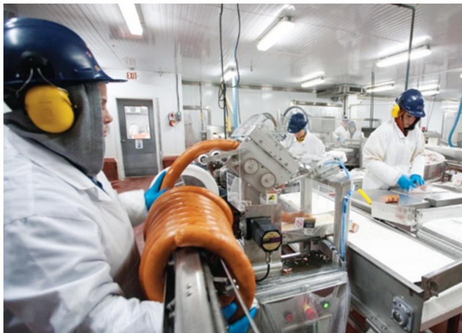
Placing a ring of sausage on a coil portioning machine, the portioner cuts sausage at a pre-determined length, corresponding to the desired product weight, prior to conveying it to the vacuum-packing lines.
