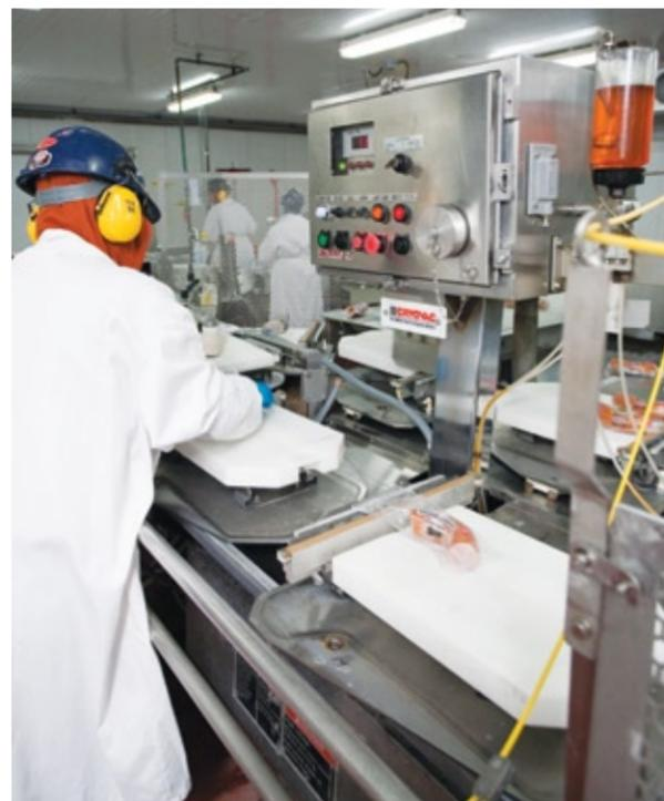
A Brandt Meat operator ensures the placement of the chub-filled bag falls properly onto the Cryovac sealing bar prior to it entering a chamber to evacuate the air and securely vacuum-seal the package.
