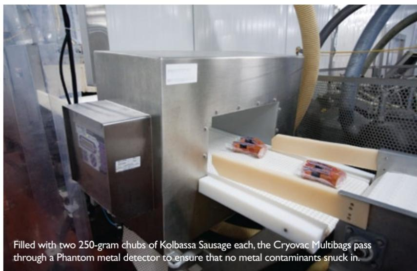
Filled with two 250-gram chubs of Kolbassa Sausage each, the Cryovac Multibags pass through a Phantom metal detector to ensure that no metal contaminants snuck in.
