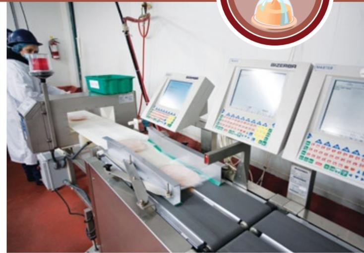
A CFS packaging line for sliced meats conveys packaged product on to a Bizerba scale to ensure proper weight prior to shipping.
