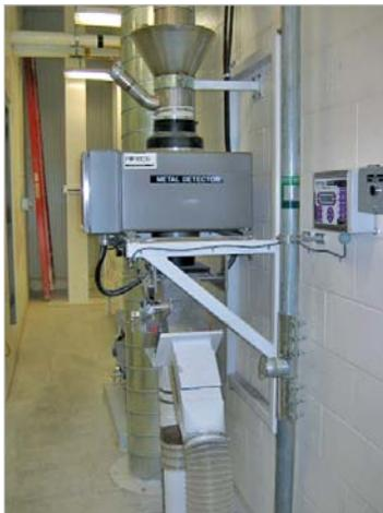
One of five Phantom Gravity metal detectors used to detect metals in free-flowing oat products before packaging.
