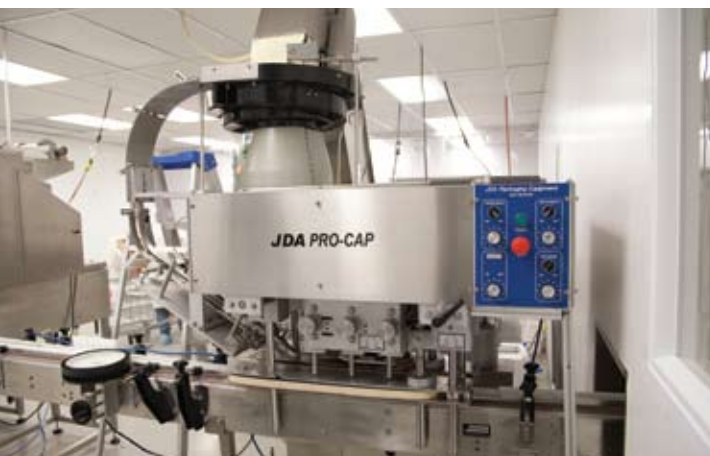
One of the two packaging lines inside the 10,000 Class cleanroom uses a JDA Pro-Cap 5000 capper for packaging candies inside metal tins and containers.
