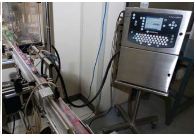
Packages of candy whisked from the 10,000 Class cleanroom pass by the Domino A100+ inkjet coder for quick printing of all the required product codes and data.
